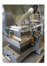
resulting in packaging line shut down until the loose capsules are cleared. In some extreme cases, the loose capsules progress into the thermoformer and cause lengthy downtime. Static electricity generation on the capsules was thought to be the reason for this issue.
